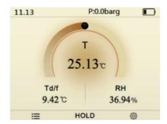
Use the arrow keys to change the appearance of the measurement window. Two different versions are available.
